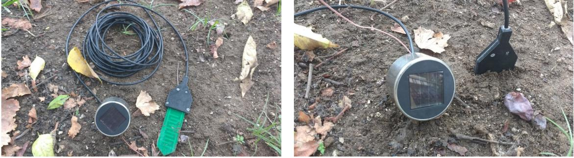
Figure 4.26: Current prototypes of FM remodulation, soil moisture wireless sensors. The wireless sensors are powered using a solar panel. During the night, they can be powered using a conventional flash-light (e.g., using the flash-light of the smartphone).
