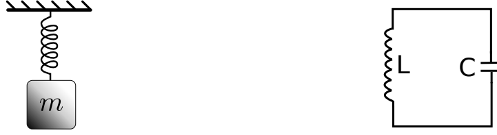
Fig. 1: Examples of systems that can be mathematically described as simple harmonic oscillators, a mass attached to a spring (right) and an LC oscillator (left).
