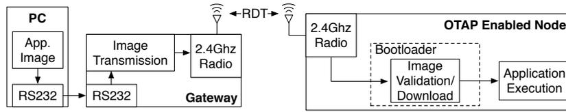
**Fig. 4.** Over the air programming block diagram.
