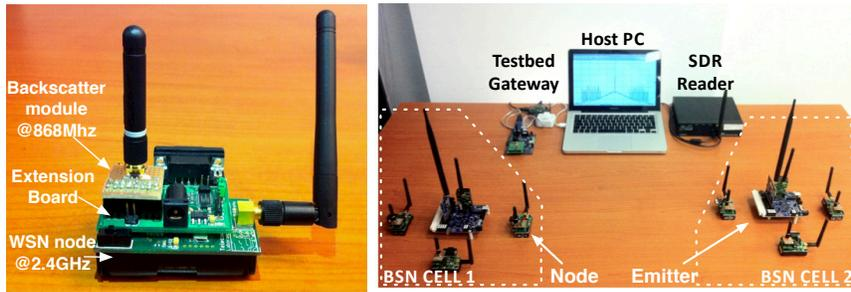
Fig. 1. Left: Hybrid testbed node. Right: Experimentation testbed.
