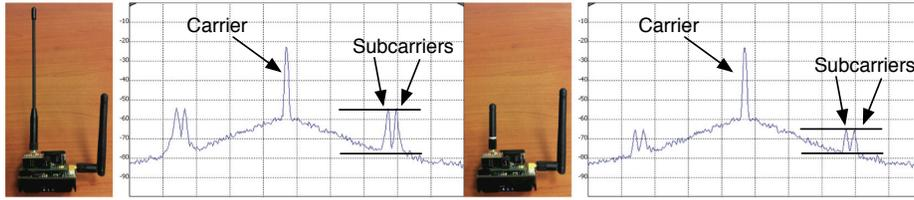
**Fig. 6.** Received power spectrum of a half-wavelength and a quarter-wavelength antenna with fixed tag-reader distance. The switching (i.e subcarrier) frequencies are clearly visible. The quarter-wavelength antenna backscattered signal has fairly smaller amplitude than the one backscattered from the half-wavelength antenna.
