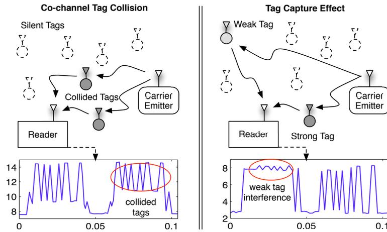
**Fig. 8.** Capture effect experimentation. Left: Tags collide by transmitting at the same time. Right: Tags are re-programmed to examine capture effect (strong tag is decoded successfully, even at the presence of a weak interfering tag). The figure depicts real signals captured by the SDR receiver.
