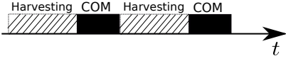
Fig. 8. Time-switching operation. Necessary energy is harvested before the communication, in duty-cycled, non-continuous applications (e.g., wireless sensors).
