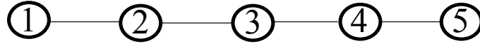
Figure 5.1: A simple PRN with 5 stations. Station 1 is one-hop-apart from station 2, while station 3 is two-hop-apart from station 1. Hence station 1, 2 and 3 cannot transmit simultaneously. With similar way we can examine which stations of the PRN cannot transmit simultaneously.
