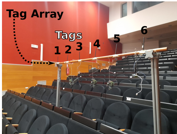
Fig. 10: Antenna array comprised of backscattering tags. The switching frequency of each tag is offered in Table I. Due to failure to achieve synchronization with the other tags during the experiments, tag #6 was omitted.
