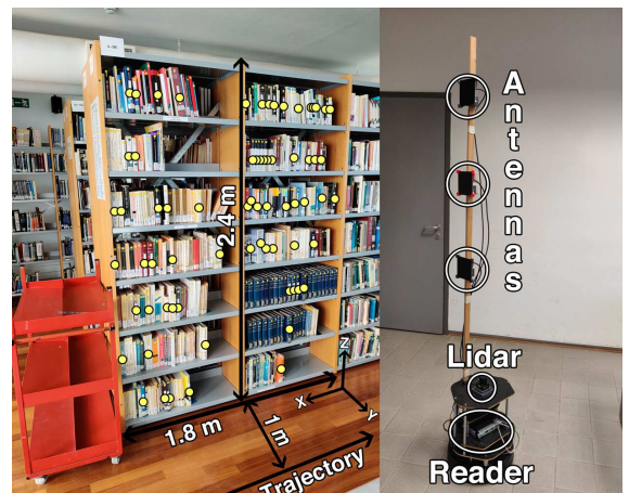
Fig. 7: Campaign 4: topology of RFID tags, trajectory (left) and robotic reader setup (right).
