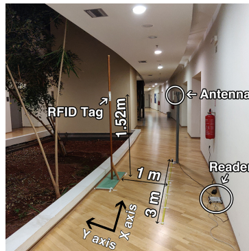
Fig. 2: Baseline experimental campaign 1: light multipath environment with manual movement of the reader antenna.
