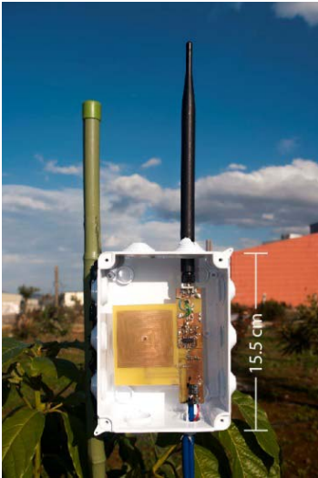
Fig. 3. Experimental prototype of the proposed self-powered wireless sensor, constructed using off-the-shelf electronic components.
