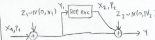
Degraded Gaussian channel.
