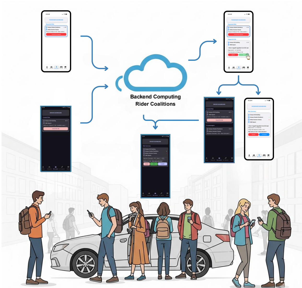
Figure 1. Match-making process overview. A passenger creates a ride request and a driver a new ride. The backend receives the data, and the match-making algorithm generates a suggested ride that the passenger receives. The passenger joins the ride and sees the ride summary. At the same time the driver receives the details of the passenger that joined. Before the ride starts, the driver receives the final passenger list, and the driver ride summary card is created.
