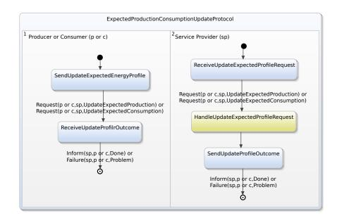
FIGURE 6.4: The model of the Update Expected Production/Consumption Protocol.
