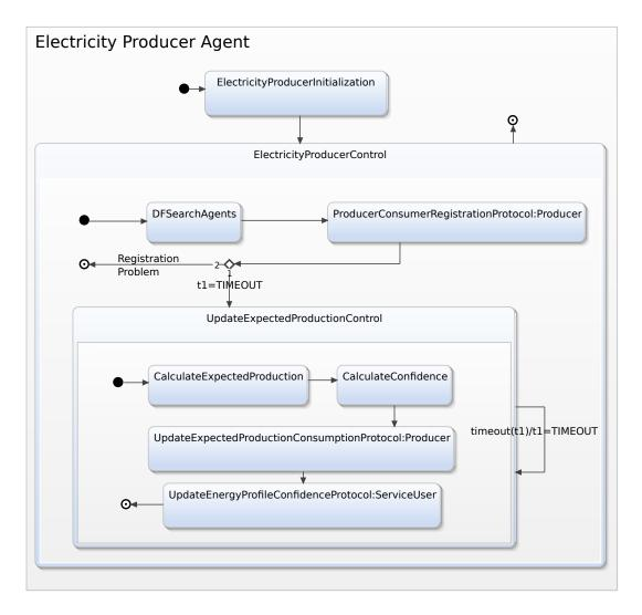
FIGURE 6.20: The intra-agent model of the Electricity Producer agent.
