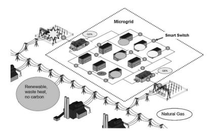
FIGURE 2.1: An overview of a micro-grid [4].
