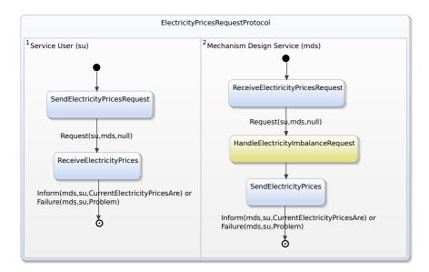
FIGURE 6.7: The model of the Electricity Prices Request Protocol.
