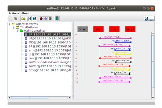
FIGURE 7.3: A screenshot of the JADE sniffer agent that illustrates the registration process and the updates of an Electricity Producer agent.
