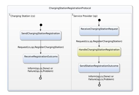
FIGURE 6.5: The model of the Charging Station Registration Protocol.
