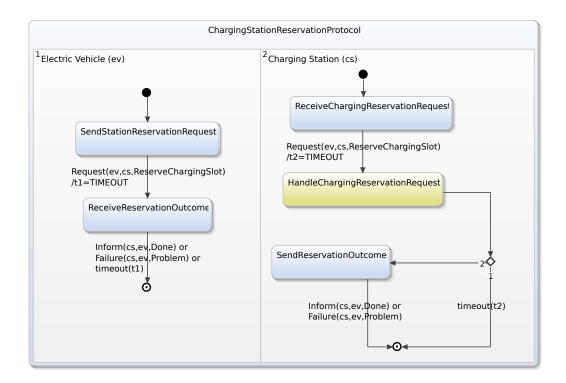
FIGURE 6.2: The model of the Charging Station Reservation Protocol.
