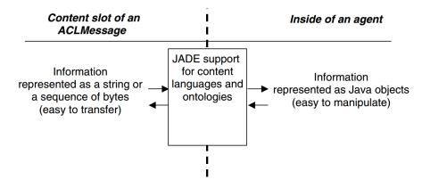
FIGURE 3.9: JADE message marshalling and unmarshalling [7].
