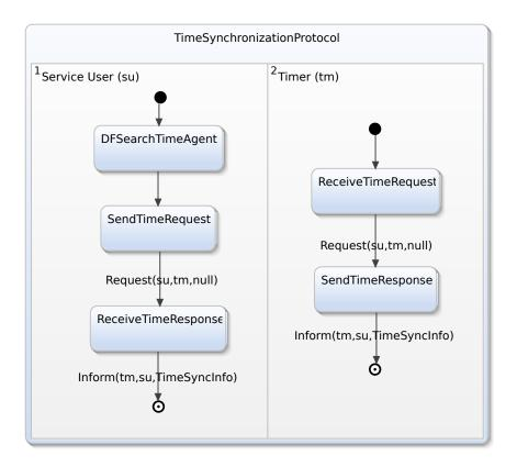
FIGURE 6.13: The model of the Time Synchronisation Protocol.
