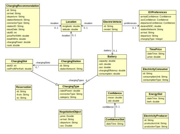
FIGURE 5.2: The concepts of the V2G/G2V Ontology given as a UML class diagram.
