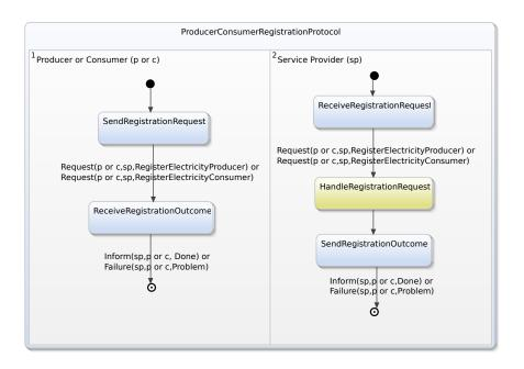
FIGURE 6.10: The model of the Producer/Consumer Registration Protocol.
