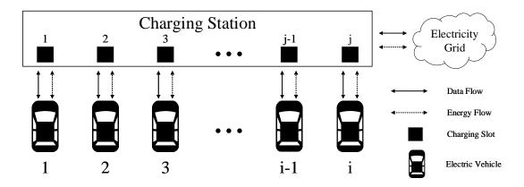
FIGURE 2.2: An overview a charging station with multiple charging slots.
