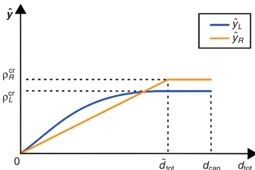
FIGURE 2 Possible functions  $\underline{\psi}(d(k))$  used to define set points  $\hat{y}(k)$  in real time at bottleneck area as function of total inflow  $d_{tot}(k)$  of motorway network.
