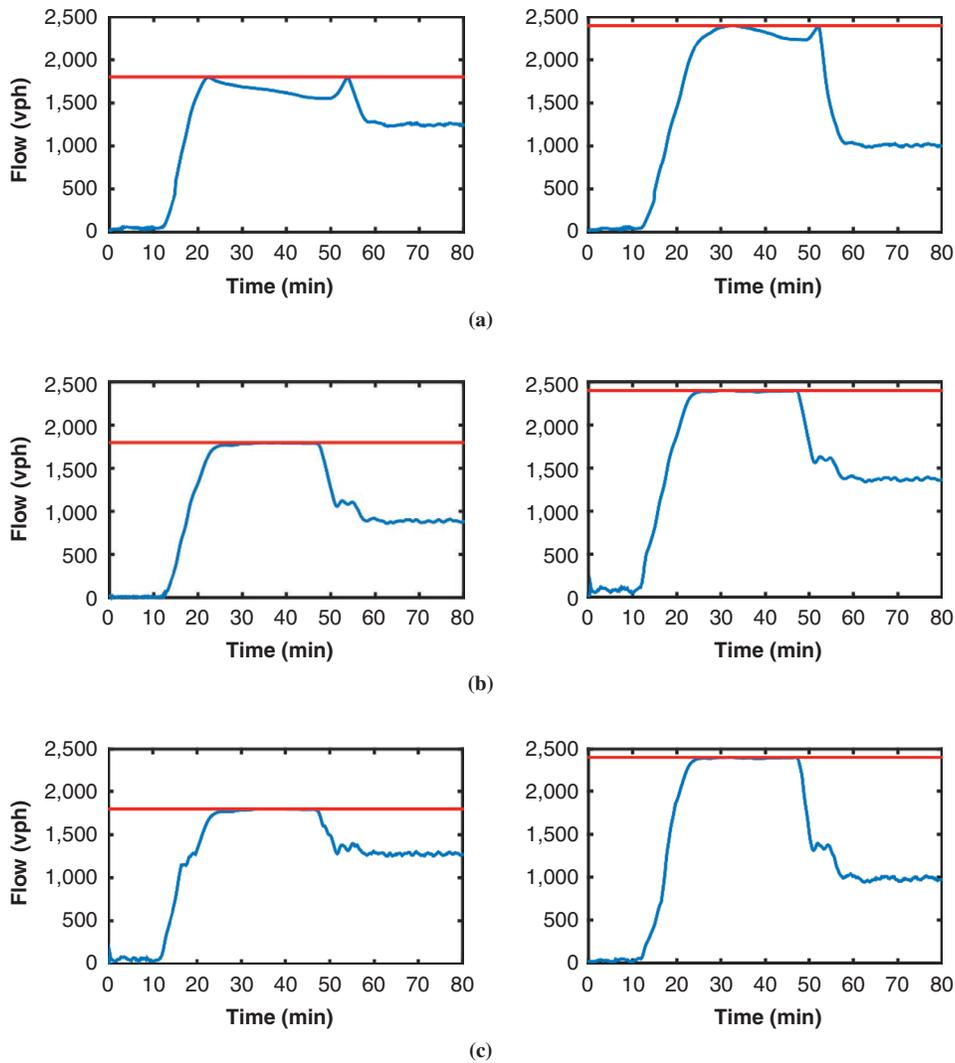
FIGURE 7 Flow exiting from Lanes 2 and 3 of Segment 5 (blue lines) and corresponding capacity flow (red lines). In (a) no-control case, capacity drop mechanism is triggered and outflow drops from capacity flow; whereas, when (b) control strategy with constant set points or (c) proposed feedback control strategy for density distribution is applied, capacity drop phenomenon is avoided and outflow during the peak period is close to bottleneck capacity.
