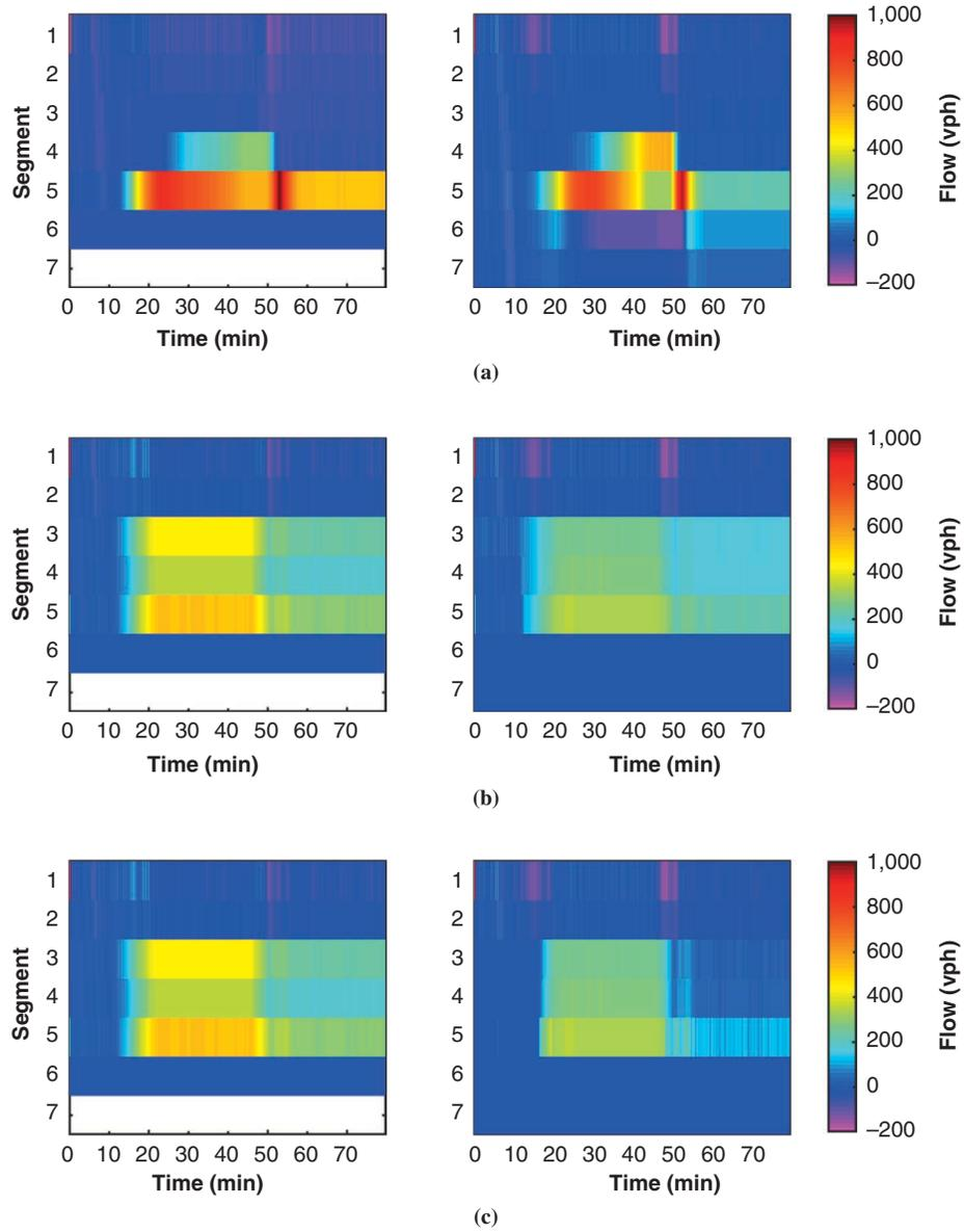
FIGURE 6 Contour plots of net lateral flows (a) in no-control case, (b) when control strategy with constant set points is applied, and (c) when proposed feedback control strategy for density distribution is applied [Lane 1 to 2 (left) and Lane 2 to 3 (right)].
