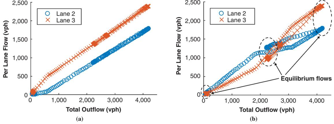
FIGURE 8 Flow exiting bottleneck area (Segment 5) for feedback control strategy (a) with constant set points and (b) for density distribution at bottlenecks as function of total outflow at bottleneck area.
