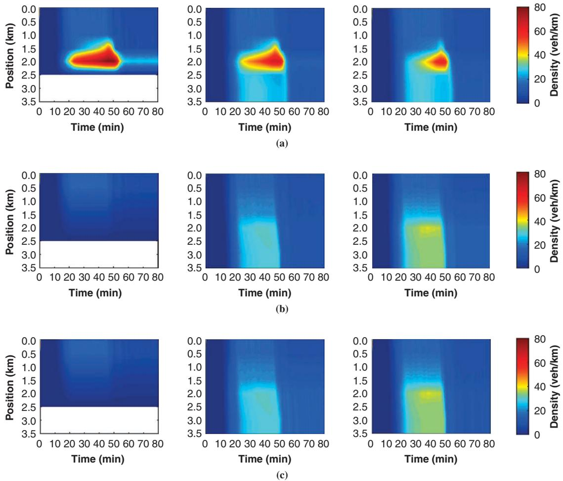
FIGURE 5 Contour plots of densities (a) in no-control case, (b) when control strategy with constant set points is applied, and (c) when proposed feedback control strategy for density distribution is applied [Lane 1 (*left*); Lane 2 (*center*), and Lane 3 (*right*)].
